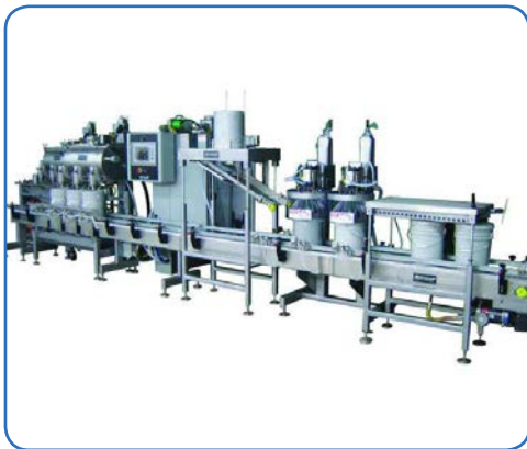
3 Head Automatic POP 3 Head Electronic Net Weight Filling Machine with Pressure Over Product (POP) Fill Cart, Crimping Station and Roller Closer for Filling Quart through 5 Gallon Containers.
