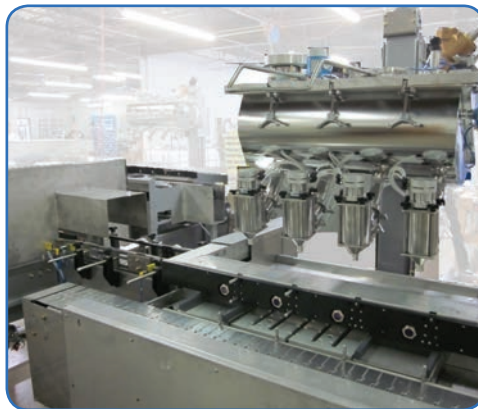
4 HEAD AUTOMATIC POP 4 Head Electronic Net Weight Filling Machine with Pressure Over Product (POP) Fill Cart and Auto Lid Placing and Closing Options.
