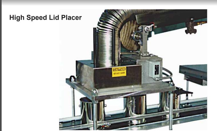
The High Speed Lid Placer is for processing up to 120 metal friction type lids per minute. The screw feed separates and continually moves stored lids into position as one is being placed. The basic unit is set up for a single size from 1/2 pint to gallons. The lid placer is adjustable to handle dimension variations of the same size lids. The optional downstacker provides 8' of lid storage.
