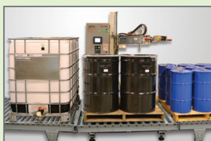
Ideal-Pak PT-IF fills a wide range of kegs, drums, totes, and pails, including 330 Gallon Plastic and 350 Gallon HDPE.
