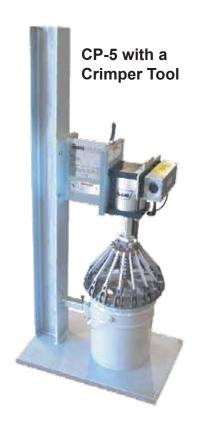
This semi automatic closing tool provides the pressure for sealing plastic and metal U.N. pails. Closing tools are easily changed with the quick release pins. The unit can be used as shown above or with a gravity roller conveyor as pictured on the back.
