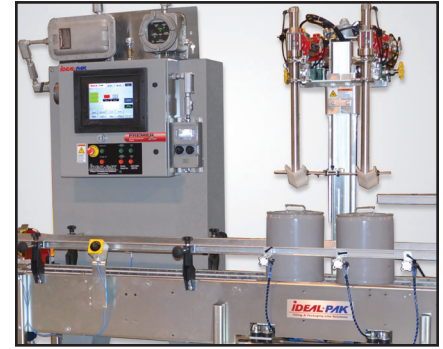
Ideal-Pak Model AE2-CNM with Manifold Cart & 2 fill lance nozzles configured for bottom filling.
