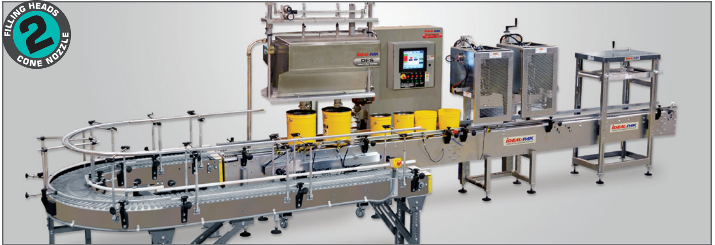
Ideal-Pak Model AE2-CGM Two Head Automatic Net Weight Liquid Filling Machine with DFS® Direct Fill System, Powered In-Feed Conveyor, 2 Gallon and 5 Gallon Crimpers (optional) and Ideal-Pak CA-NEM Heavy Duty Roller Closer (optional).
